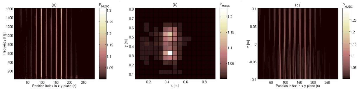
Figure 2. Music power on the source plane ( $z = 0$  m) (experiment): (a) from 0 to 1600 Hz (maxima at  $n = 98$  and  $170$ ), (b) mapped to the  $x$ - $y$  plane at 1200 Hz, and (c) as a function of  $n = 1$  to 288 and  $z = -0.1$  to  $0.1$  m (when  $n = 98$ ,  $\text{MAX}(P_{\text{MUSIC}}) = 1.298$  at  $z = -0.021$  m and when  $n = 170$ ,  $\text{MAX}(P_{\text{MUSIC}}) = 1.135$  at  $z = -0.005$  m).
