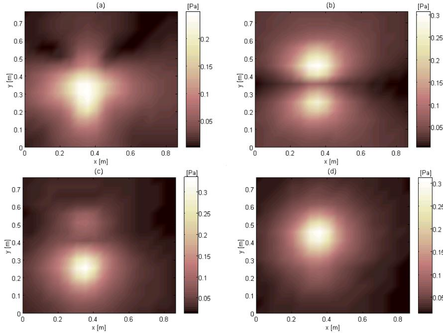
Figure 3. Amplitudes of decomposed partial pressure fields on the hologram surface at 1200 Hz when the measurement was made using references 3 and 5 (experiment): (a) 1st field (real references, PCD), and (b) 2nd field (real references, PCD), (c) 1st field (optimal virtual references, PCD), and (d) 2nd field (optimal virtual references, PCD).
