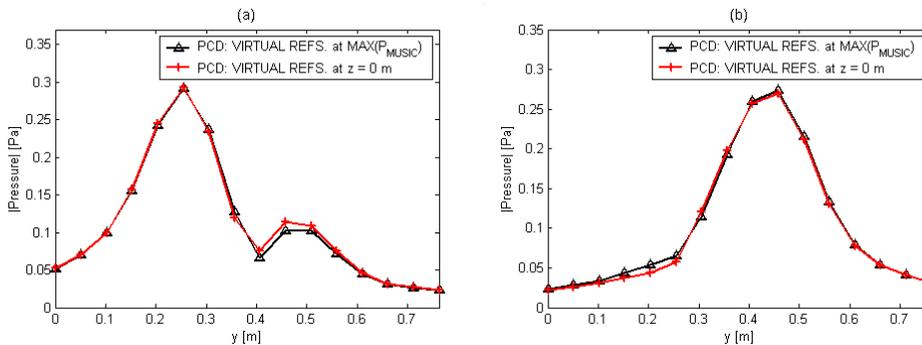
Figure 5. Amplitudes of partial sound pressure fields at  $x = 0.356$  m as a function of  $y$  obtained by using virtual references placed on source surface and at the maximum MUSIC power locations: (a) first partial pressure field, and (b) second partial pressure field.
