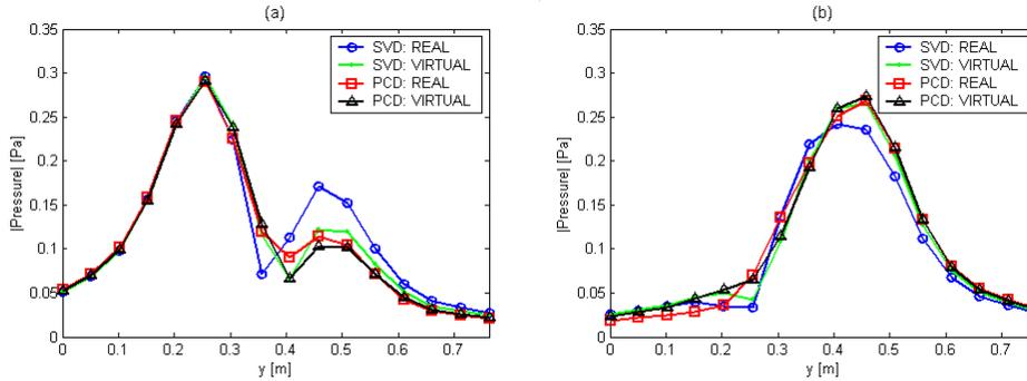
Figure 4. Amplitudes of partial sound pressure fields at  $x = 0.356$  m as a function of  $y$  obtained by using sets of real references 1 and 2 and optimal virtual references: (a) first partial pressure field, and (b) second partial pressure field.
