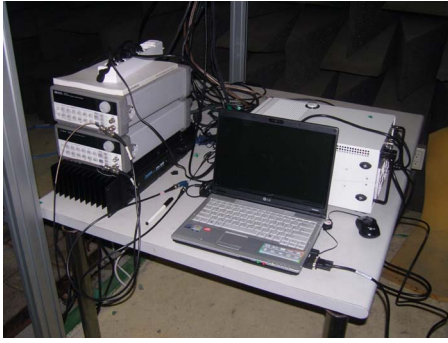
FIG. 4. (Color online) Photo of experimental setup: two HP signal generators, two-channel loudspeaker amplifier (in black), NI data acquisition system, and laptop.
